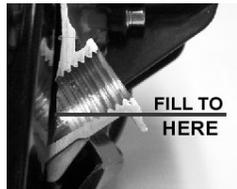
4. Turn oil-fill cap counter-clockwise and remove cap from oil-fill opening. Proper oil level should come to the middle of the threads in the lower part of the oil fill hole, as pictured above.
